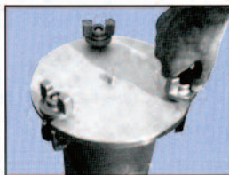
1. Unscrew 3 hand knobs and pivot knobs away from cover.
