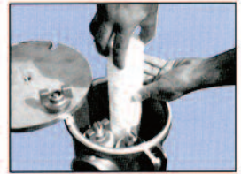
5. Drop in new tubes, replace tube cap nuts and secure cover.
